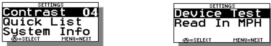
**Contrast** – To adjust the darkness of the lettering on the screen you can change the contrast. This value can be adjusted from 0-10 and is saved in the memory. The smaller the number, the brighter the screen will be in bright sun.
