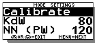
**Calibrate** – Used to calibrate the PerfectPass digital speedometer readout. The procedure for adjusting this can be found in the *Section 7: Digital Speedometer Calibrate*. The calibration screen can also be accessed from the Main WAKEBOARD Screen by pressing the **DOWN** key with the
