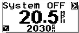
**Engaging System** – With PerfectPass ON, the system will automatically engage once the **SETPOINT** is reached. PerfectPass requires the driver to bring the boat up to and slightly past the **SETPOINT** before it will engage. When the system engages it will sound an audible beep and the top line will become highlighted. In Slalom mode the screen appears as follows:
