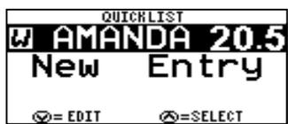
**Creating Names** – First enter the Name List. Press the **MENU** key until [NEW ENTRY] is highlighted. Then press the **UP** key to enter a new name. The following screen will then appear:
