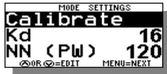
**Calibrate** – Used to calibrate the PerfectPass digital speedometer readout. The procedure for adjusting this can be found in the Digital Speedometer Calibrate Section 7, Page 19. The calibration screen can also be accessed from the Main Trick Screen by pressing the **DOWN** key with the
