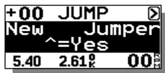
*Press the UP key to enter a new jumper or DOWN key to enter or edit the crew weight. New Jumper is covered below.*
